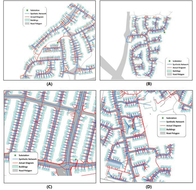
Figure 5: example comparison of (A) detached, (B) semi-detached (duplex), (C) terrace (townhouse), (D) mixed building layouts
