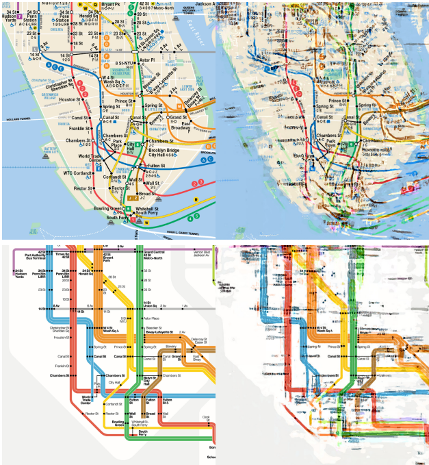
Figure 19: Computer modelling by Ruth Rosenholz of peripheral vision information attenuation for two different New York City Subway maps: Official MTA topographical design (top), MTA weekend map (bottom). In each case the visual focus is Canal Street. Thin lines with complex trajectories are particularly vulnerable. For example, on the topographical map, the lines almost disintegrate as they head northwards through Manhattan [Ros11].
