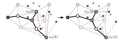
Fig. 7. An exemplary move swapping the assignments of customers k and l.
