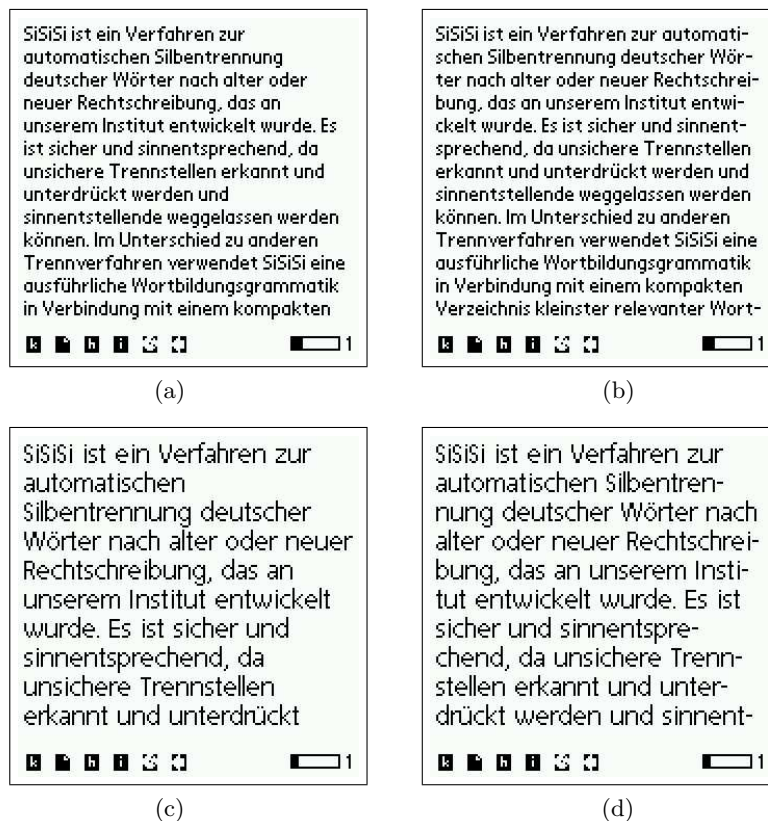
Fig. 5. The same text as displayed by PalmReader on a PDA screen using the small font (a) without and (b) with pre-hyphenation, and the large font (c) without and (d) with pre-hyphenation, respectively. Note that (b) and (d) show the identical pre-hyphenated file, but different soft hyphens are being used for actual end-of-line hyphenation.
