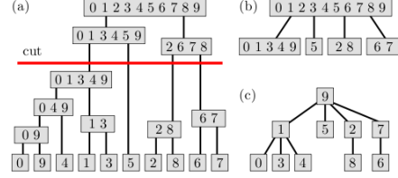
Figure 2: Hierarchical clustering (a), height-restricted clustering (b), and the resulting diameter constrained tree with D = 4 (c) after choosing a root for each cluster in (b).
