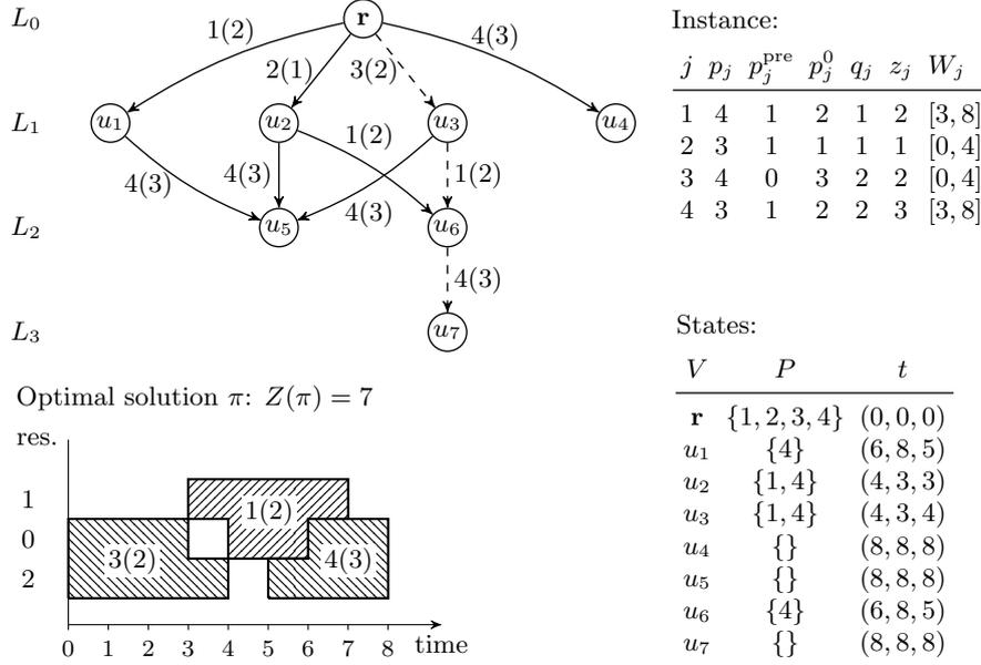
Figure 1: A MDD for an example instance with four jobs and two secondary resources.
