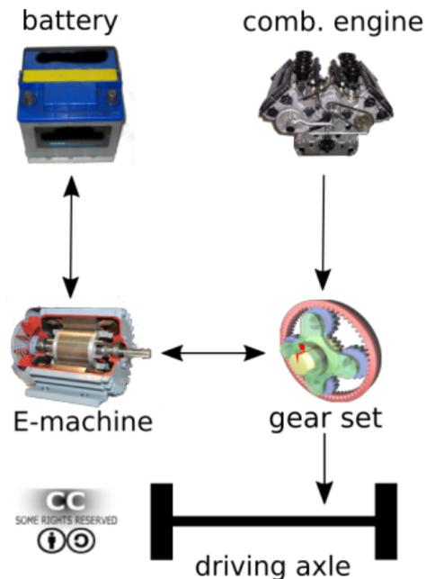
Figure: Structural HEV scheme
